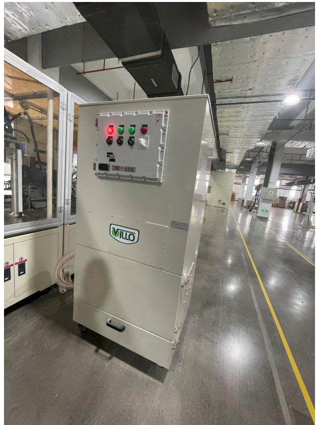
焊接烟尘滤筒除尘
